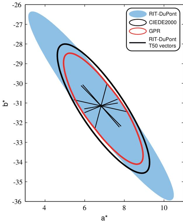
**Figure 5.** RIT-DuPont color center 17 projected on the CIELAB  $a^*b^*$ -plane. Suprathreshold ellipsoid (blue) fitted to the RIT-DuPont T50 and -T50 vectors compared to CIEDE2000 iso-distance contour (black) and GPR-based iso-distance contour (red). STRESS values: CIEDE2000 4.50, GPR 2.41.
