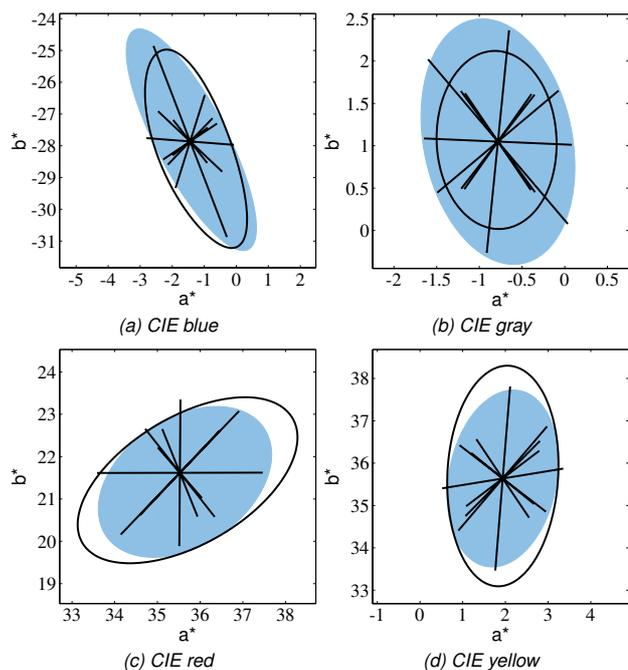
**Figure 1.** Four color centers recommended by the CIE for study [17]. RIT-DuPont suprathreshold ellipsoids (blue) with the corresponding T50 and -T50 color-difference vectors in comparison with CIEDE2000 iso-distance contours (black). Each point on a contour has a computed distance of 1 to the respective color center. Projections on the  $a^*b^*$ -plane.
