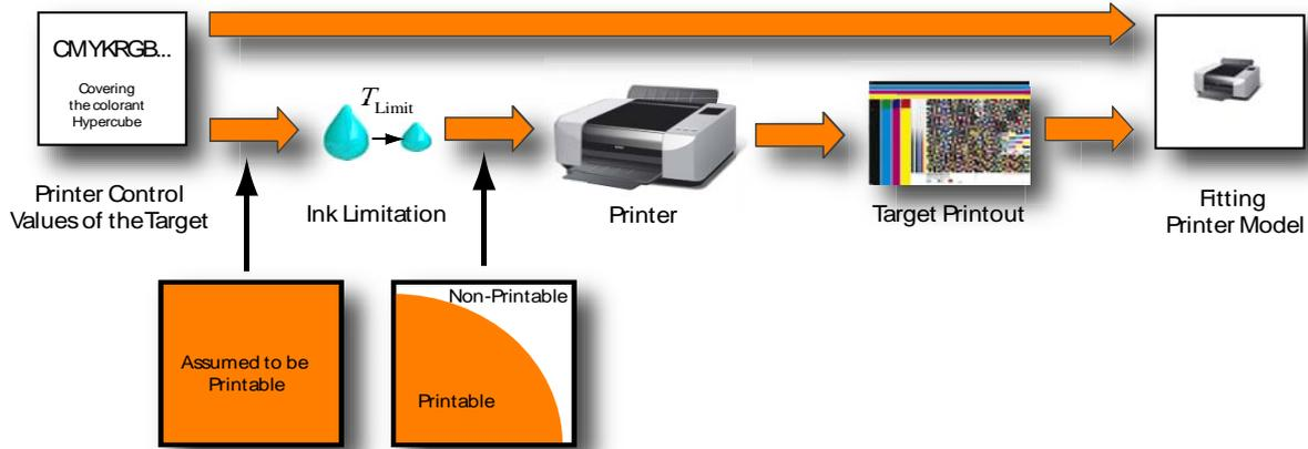
Figure 3: Ink limitation is performed before the target data is send to the printer. The printer model is fitted to the target printout and the non-ink limited control values.
