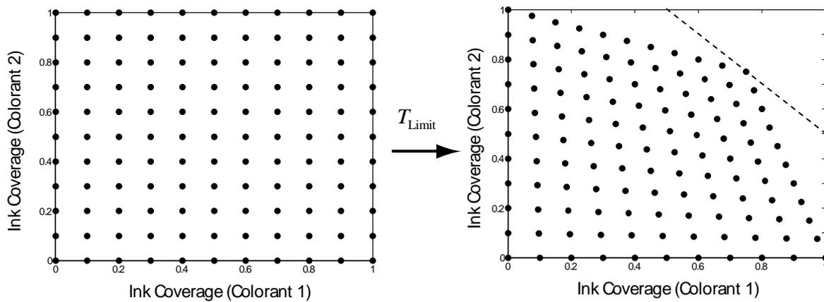
Figure 5: Example of the multi-linear transformation for a printer with two colorants and  $\psi_{\max}=1.5$ .
