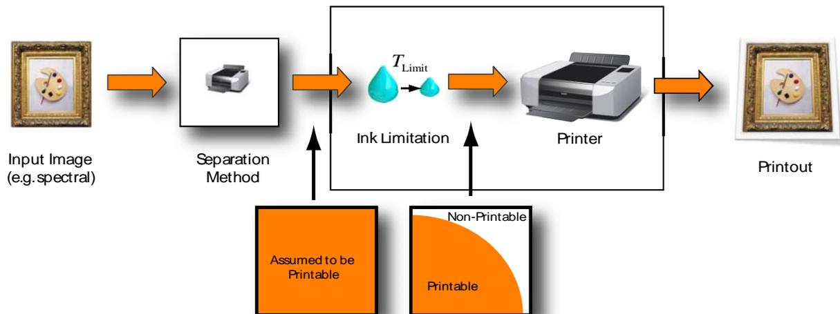
Figure 4: General printing workflow: Ink limitation is treated by the separation method as part of the printer.
